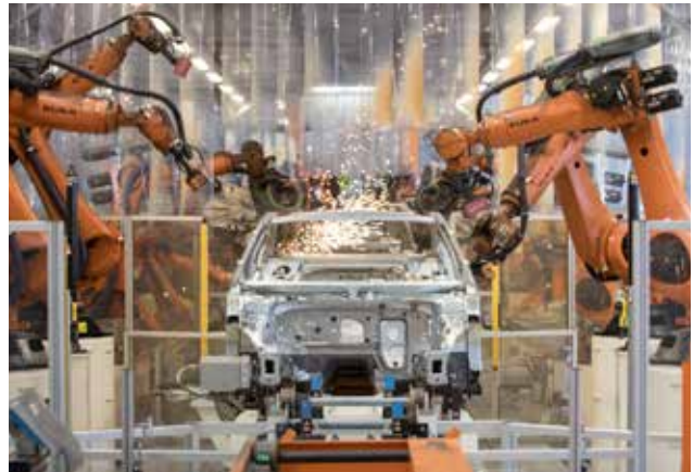
Robots assemble parts of a vehicle at the Volkswagen plant in Emden. Accounting for 15.5% motor vehicles and parts thereof of exports, was Germany's main export product in 2020.
